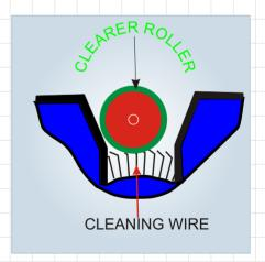
The bottom roller is having straight nylon bristles and these engage with the metal wires of top roller so that the waste collected by top roller is completely discharged by the bottom roller and the waste is collected at the bottom chamber of the machine.
